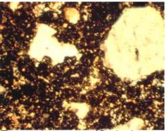
The granular structure of Portland cement Expérimentales sur la surrounding sand explains its weakness Chaux de Construction, because the structure is not compact.
