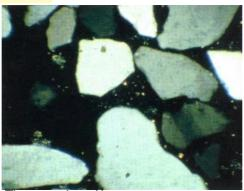
The smooth and homogenuous structure of Geopolymer cement surrounding sand.
