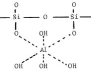
On the other hand, Me-silico-aluminates, where Me is a metallic cation, like Na, K, Ca, etc, are salts of the aluminium hydroxide side groups branched to a silicic acid backbone that is to say, of a silico-alumino acid. Here,  $AI^{3+}$  is in 4-fold coordination with O and OH as in aluminate ions  $AI(OH)^{-}$
