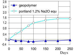
Figure 7: Alkali-Aggregate Reaction; ASTM C227 bar expansion test on PZ-GEOPOLY® Geopolymer cement and ordinary Portland Cement.
