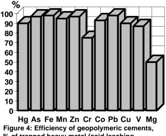
Figure 4: Efficiency of geopolymeric cements, % of trapped heavy metal (acid leaching, constant pH 5, Reg. 309), Potassium-Poly(sialate-siloxo) K-PSS type
