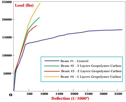
Figure 3: Load vs Deflection. All Beams
