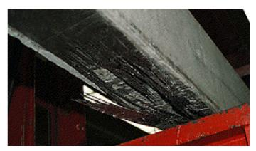
Figure 5:Rupture of Geopolymer-Carbon composite
