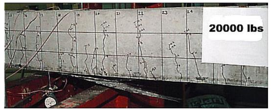
Figure 4: Cracking Pattern for Beam # 2 at 20000 lbs Load, after Rupture of Composite (bottom)
