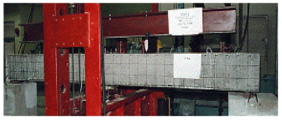
Figure 2: Beam Prior to Start of Testing
