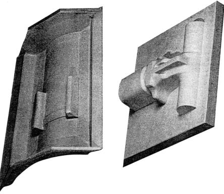
Figure 6: Autoclave and press molding tools made of castable F,M-PSDS Geopolymite resin and corundum aggregates with tailored grain size for Gel-Coat and core.
