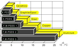
Figure 3: Coefficient of Thermal Expansion for geopolymers and tooling materials
