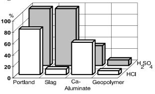
Figure 1: Break up in 5% acid solutions (% of matrix dissolved under identical conditions) [21,
