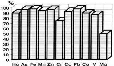
Figure 1!: Amount of hazardous elements locked in the geopolymeric matrix.
