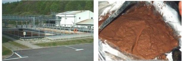
Figure 4: The water treatment plant at AUE Schlema-Alberoda. The geopolymeric waste material was poured in big-bags, ready for disposal.
