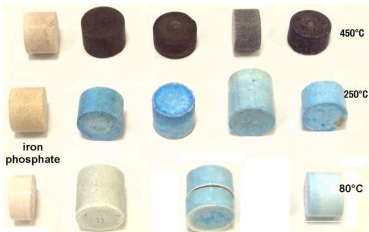
Figure 5: heat-treatment above 350°C transforms turquoise-blue into black CuO, tenorite, with the exception of iron-phosphate that remains beige.
