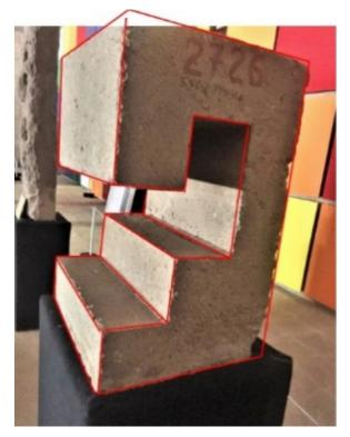
Figure 14: Tiahuanaco Lithic Museum: lithic sculpture made easily with geopolymers, interior and exterior right angles, flat surfaces.
