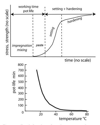
Figure 10: Top, the four phases of geopolymerization: working time / pot life / setting / hardening; bottom, pot life for K-poly(sialatedisiloxo) resin and storage temperature (Davidovits, 2008-2020).
