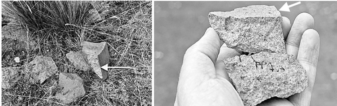
Figure 21: Left, andesite monument fragments (debris) lying on the ground, the arrow points on the fresh broken part source of the PP1 sample; right, PP1 A and B with the smooth finish and perfectly flat face (white arrow), after [2].
