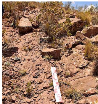
Figure 11: MAR sampling site of weathered, easily disaggregated sandstone layers.
