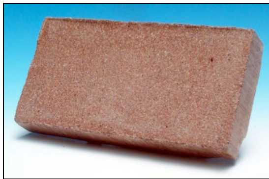
Figure 5: Brick made with L.T.G.S. on kaolinitic soils. Mechanical compressive strength in Mpa for untreated and geopolymerised kaolinitic earth (with 3% by weight equivalent Na 2 O). Setting temperature ranges between 20°C and 1000°C.
