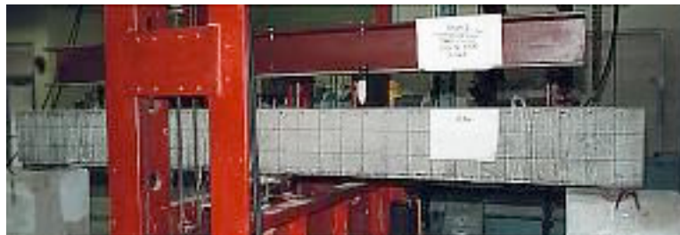
Figure 15!: Concrete beam (3 meters long) with Geopolymer Carbon composite layers applied on its bottom surface, before testing
