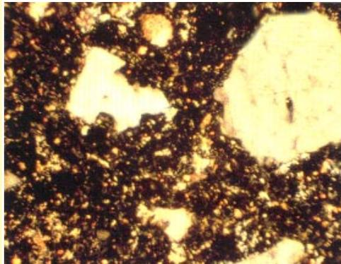
The granular structure of Portland cement surrounding sand explains its weakness because the structure is not compact.
