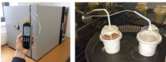
**Figure 4:** Reactivity test, observing exothermicity, oven at 80 °C.
