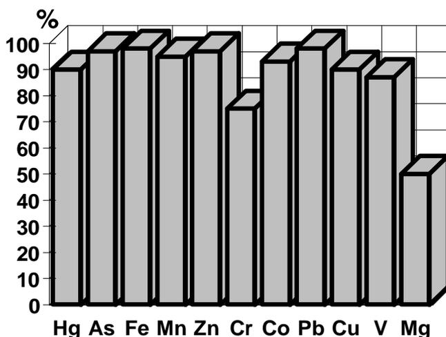
**Figure 4: Efficiency of geopolymeric cements, % of trapped heavy metal (acid leaching, constant pH 5, Reg. 309), Potassium-Poly(sialate-siloxo) K-PSS type**
