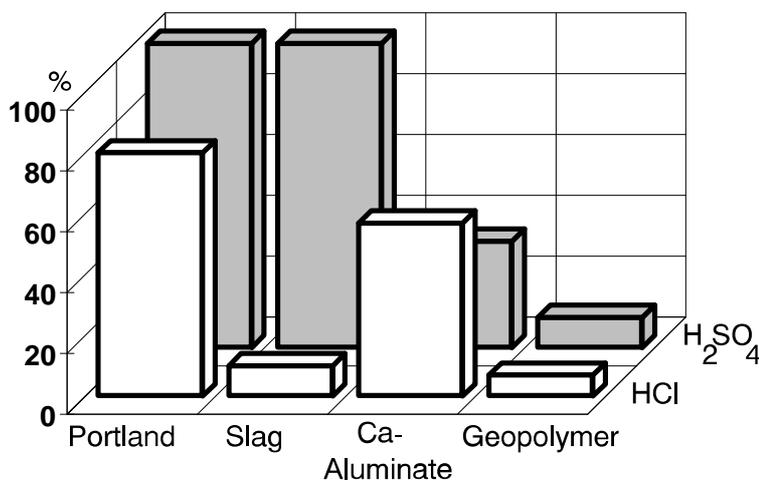
Also, the binding matrices control the maximum credible concentrations of hazards in the leachates, and keep them below known health effect levels. In addition, geopolymer monoliths can hold the hazards below the detection limits of analytical methods.
