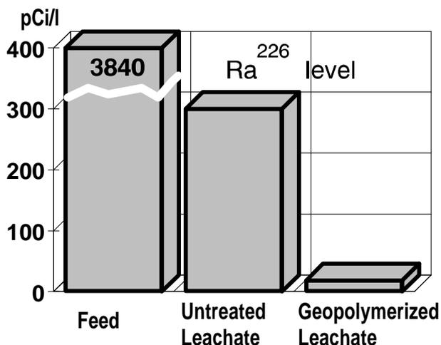
**Figure 3: Radium level in uranium waste tailing (acid leaching, constant pH 5, Reg. 309), Potassium-Poly(sialate-siloxo) K-PSS type GEOPOLYMITE® binder.**
