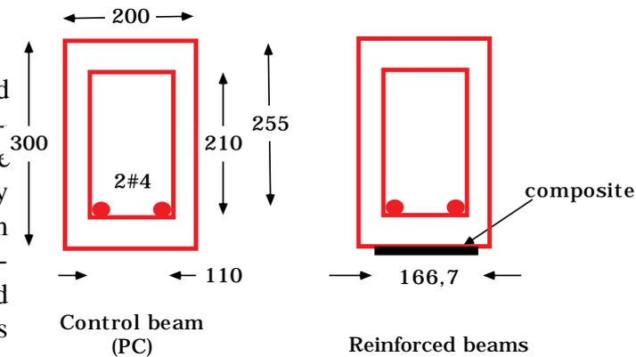
Figure 1: Beam Cross Sections
