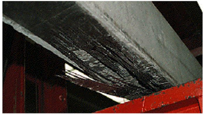
Figure 5: Rupture of Geopolymer-Carbon composite
