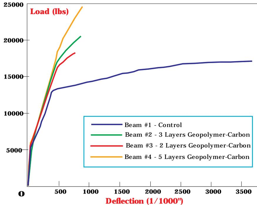
Figure 3: Load vs Deflection. All Beams
