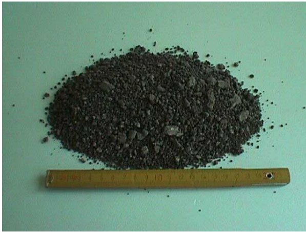
Granular pre-product (Sludge + P.C.) after hardening
