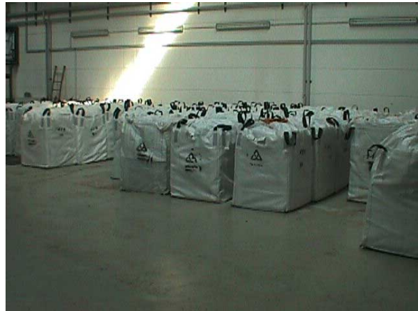
Demoulded Big Bags with hardened blocks
